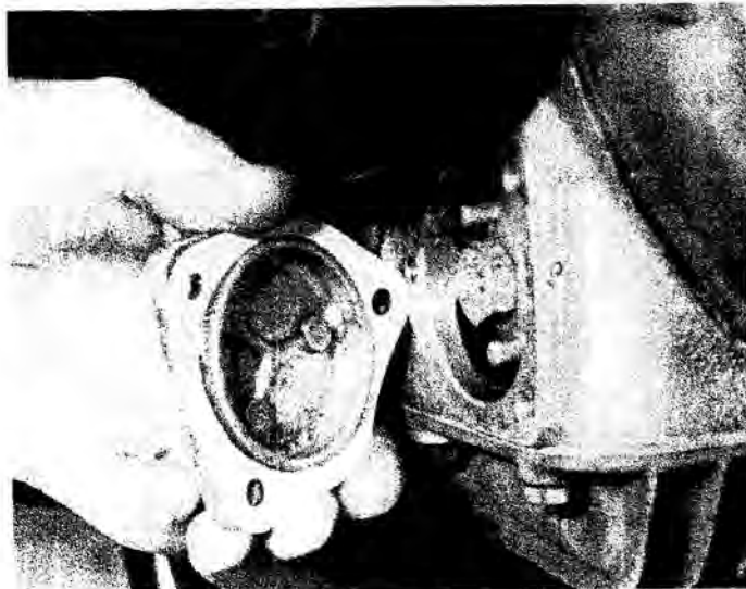
Ensure that all gaskets and O-rings (where fitted) are renewed before refitting filter cover
