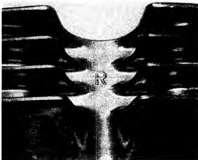
Note cast marks identifying left- and right-hand rocker covers – later models only
